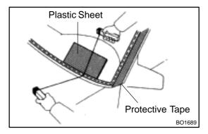
(c) Cut the adhesive by pulling the piano wire around it.
